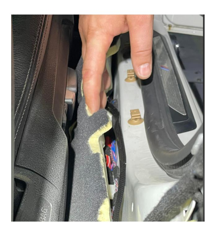
Harness is being routed to this area where the BDC (FEM) unit is located:
