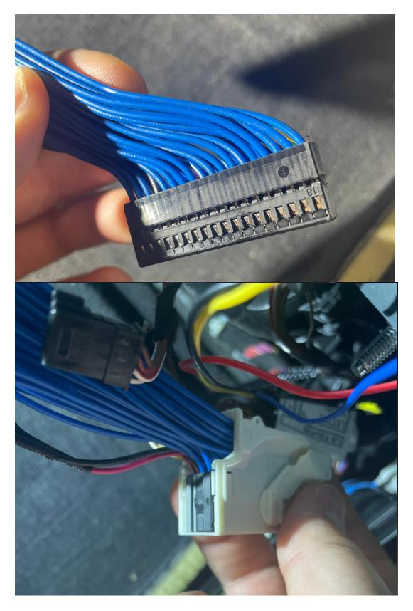
Slide the large white connector back into the BDC (FEM) CON7 location and ensure it is locked back into place with its latch as shown in picture below.
