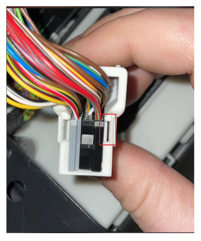
Insert the blue harness connector in place of the OEM black sub-connector:
