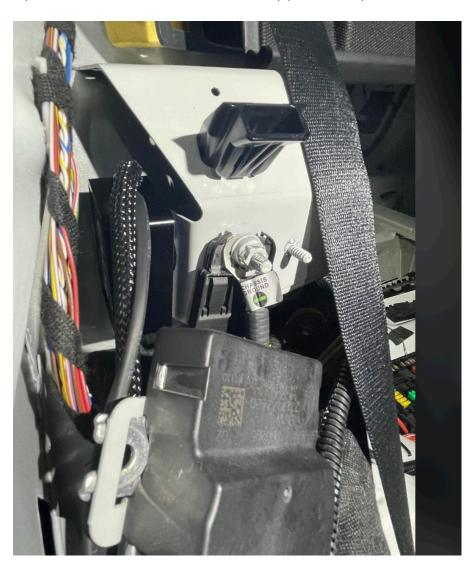
The only difference in this case is that the long harness is now being routed to the passenger side footwell area to the vehicle's FEM (BDC) unit.
