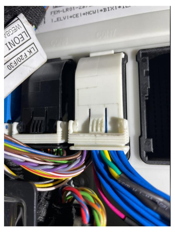
Connect the other side of the blue BM3 harness to the OEM black sub-connector as shown in picture below.
