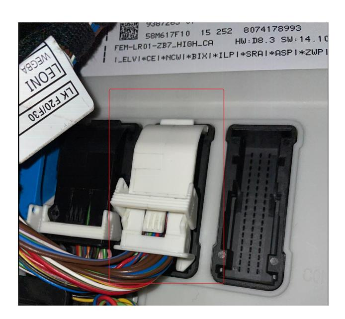
Unplug it and pull out the black sub-connector by pushing the small tab on the right outwards and pulling the black sub-connector out.
