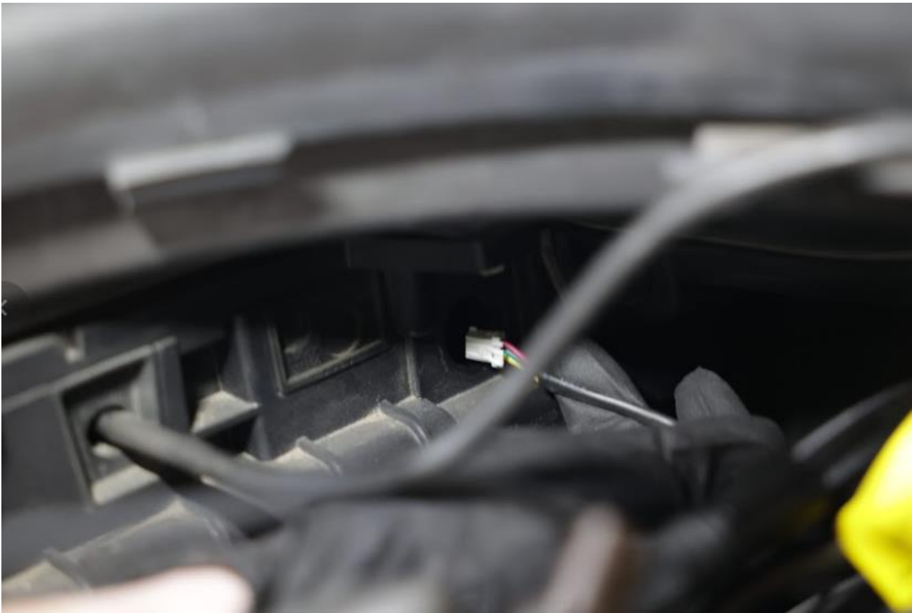
25. Connect sensor 3 pin wire harness (black connector) to the bootmod3 flex fuel kit housing
