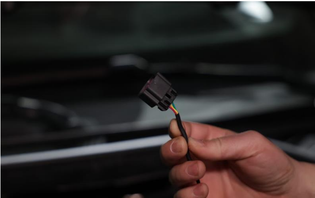
25. Connect sensor 3 pin wire harness (black connector) to the bootmod3 flex fuel kit housing
