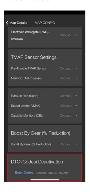
We have added a new feature to enable users to selectively remove DTCs (Diagnostic Trouble Codes) on maps. In the cases of extensive hardware modifications, relating to the engine or its accessories, there are times when its nice to turn off certain codes from coming up.
