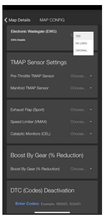
Electronic Wastegate (EWG) is one of our new features. Customers going with aftermarket big turbo kits there the factory EWG controller is being removed in favor of the conventional wastegate (e.g. Tial, Tubrosmart, etc.) for boost control. EWG OEM set up is great but this option makes it much easier for custom tuners to dial in the big turbo set up and focus on what matters the most, making gains.
