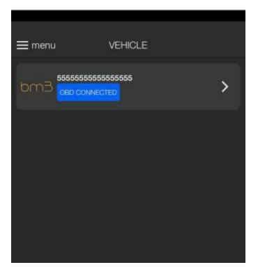
Once the connection with the car has been established, the red box will turn blue and it will say "OBD CONNECTED".
