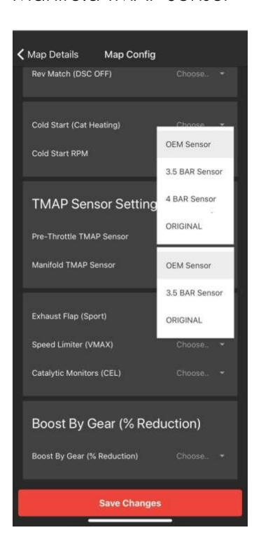
Users may wish to change the Pre-throttle and Manifold TMAP sensors on certain vehicles where the boost will exceed factory TMAP sensors, typically with custom tunes. Only change these settings if certain of the changes. If the changes don't match the sensor after flashing the map the vehicle will stumble, get a drivetrain malfunction and won't idle.
