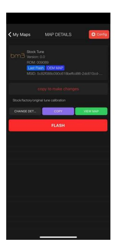
Stock Factory Tune is automatically created for the vehicle upon activating the license. Factory tune is based on the software details on the vehicle's DME. Flashing to stock tune is always an option. This is typically done when a license transfer needs to be completed. Other times include; if the vehicle needs to be taken to the dealership or simply if there is no more desire to drive with the OTS map.
