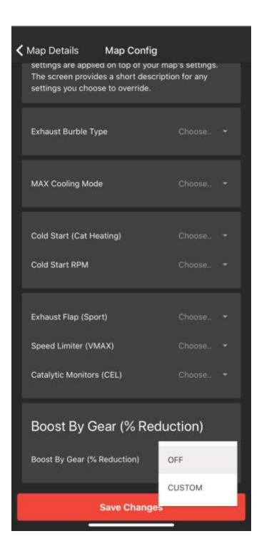
Many people on the racetracks can attest to having traction issues, especially in lower gears. These issues are about cutting better 60' at the ¼ mile or in a 2nd gear roll, given how torque ramps in quickly on these cars. This is a great feature we have added where user can reduce the boost by gear to their personal liking. Quality tires and proper suspension set up go a long way.
