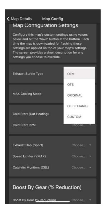
Exhaust Burble is one of **bootmod3's** most desired features. It enables the user to customize the exhaust burble to personal liking. There are five choices to select from.
