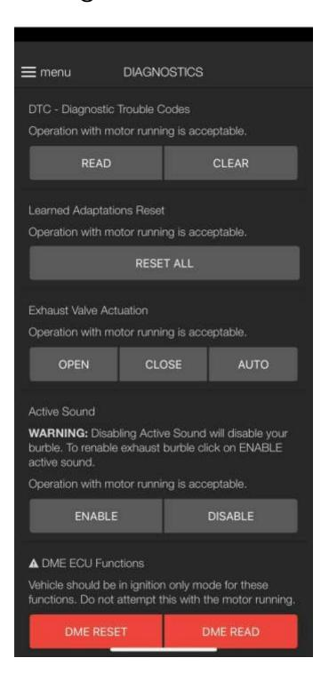
The Diagnostics screen is mainly used to read codes from the DME.
